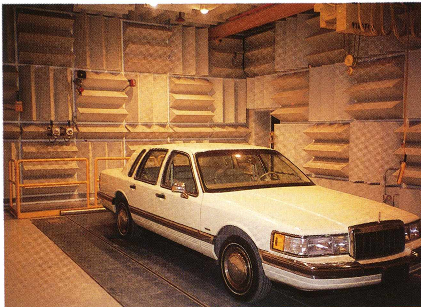
One of ten Hemi-Anechoic Rooms with Metadyne Wedges at Advanced Engineering Center, Ford Motor Company, Dearborn, Michigan. Specifications required cut-off frequencies of 125 Hz, 90 Hz, and 60 Hz.
