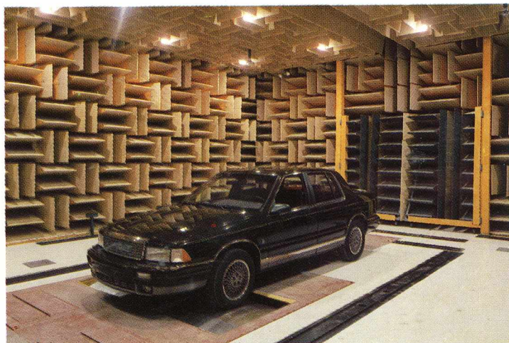
One of three similar sized IAC Hemi-Anechoic Rooms, with glass-fiber wedge cut-off frequencies of 90 Hz, at Chrysler's new Tech Center, Farmington Hills, Michigan. Albert Kahn were the Architects and Walbridge Aldinger, Construction Managers.
