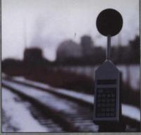
Handheld Sound Level Meters Measuring, Logging, Monitoring 110 dB dynamic range, AC output
