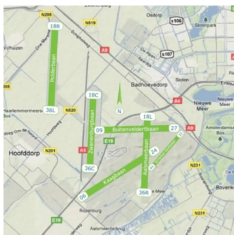
Fig 2. Lay-out of AMS. In 2000 runway 36L-18R was added. The smaller 04-22 runway is for general aviation only.
