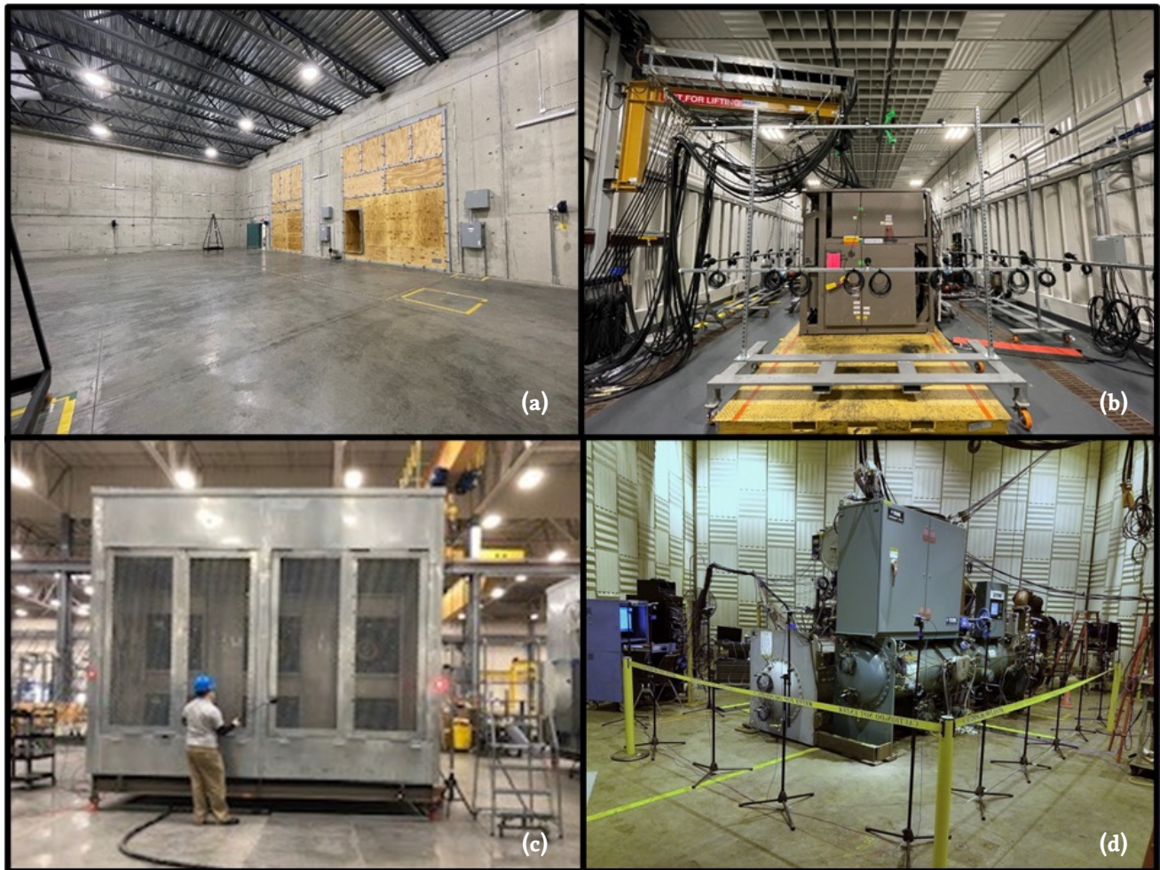
Figure 1: (a) Reverberation room used for testing HVAC equipment in accordance with AHRI 220 (b) Microphone grid for sound testing air-cooled chiller in a free-field according to AHRI 370 (c) AHU testing using sound intensity in accordance with AHRI 230 (d) Microphone grid for sound testing water-cooled chiller in a free-field according to AHRI 1280. Photos Courtesy of Johnson Controls
