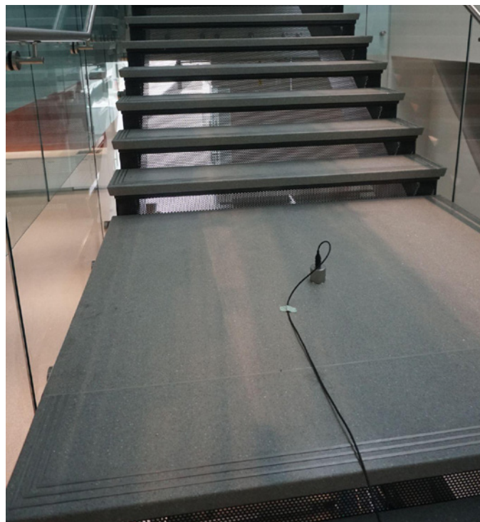
Figure 4. Vibration testing with accelerometer at intermediate landing.
