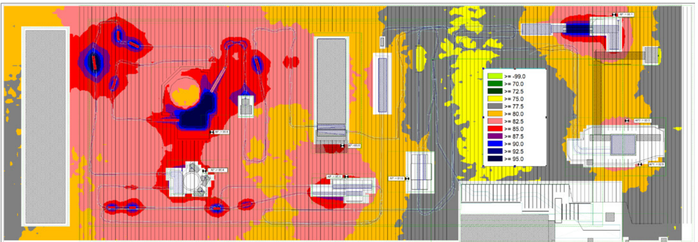
Figure 3: Variant A-weighted level map with baffle ceiling, showing reduced levels over larger areas due to a lower diffuse sound field component.
