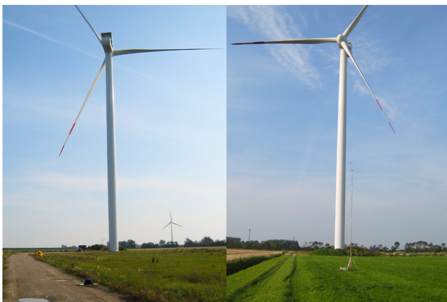
Figure 2: Photos from a measurement. Left: Photo of the microphone under a secondary wind screen on a plate on the ground. Right: Photo of a meteorology mast used for determining the wind speed during background noise measurements.
