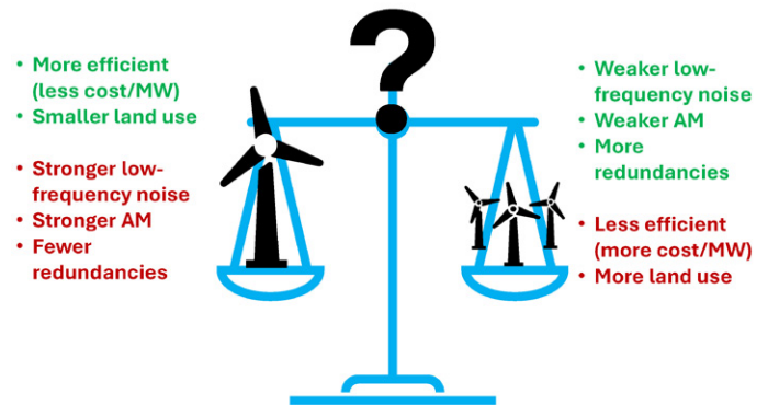
Figure 3 - Conceptual comparison of two wind farm layouts with equal energy production: a few large turbines (left) vs. many smaller turbines (right).
