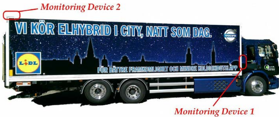
Figure 1. Position of the microphones for the noise-monitoring devices mounted on the trucks. "We run hybrid electric in the city, night and day."
