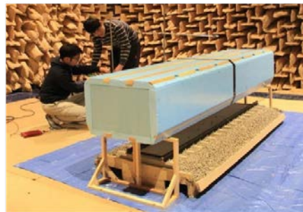
Figure 10: Investigations of the effect of the vehicle on rolling noise. Upper: boundary element model; Lower: 1:5 scale model tests (ISVR)
