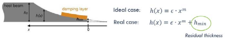
Figure 12: Effect of residual thickness in an ABH. Schema from Pelat et al. / Journal of Sound 22 and Vibration 476 (2020) 115316
